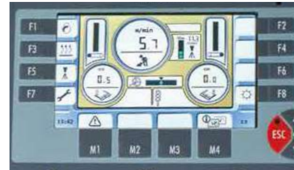
Indication of maximum pave speed The display shows the maximum possible pave speed which still ensures full coverage of the road surface.
