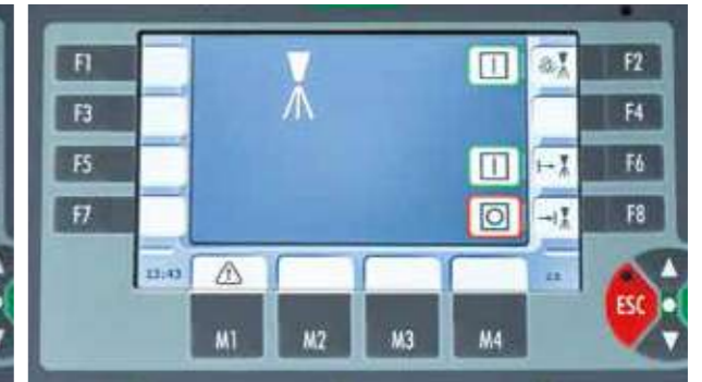
"Start of Job" and "End of Job" The convenience functions "Start of Job" (F6) and "End of Job" (F8) are provided so that spraying always starts and ends at exactly the required point and continues over full pave width.
