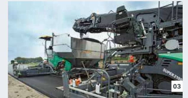
By way of the transfer module on the paver placing binder, surface course mix is conveyed to the second paver following behind.
