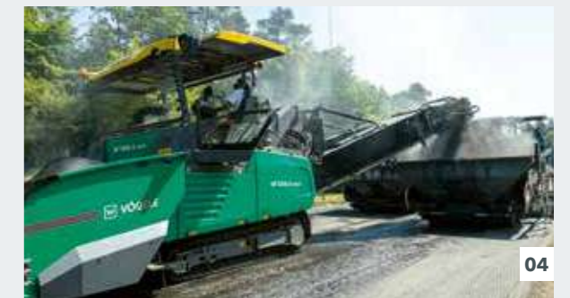
The feeder operator has an unimpeded view of the feed vehicles and the SUPER 2100-3i IP.
