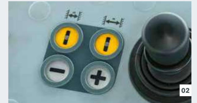
For automatic distance control the operator can select between two different distances.
