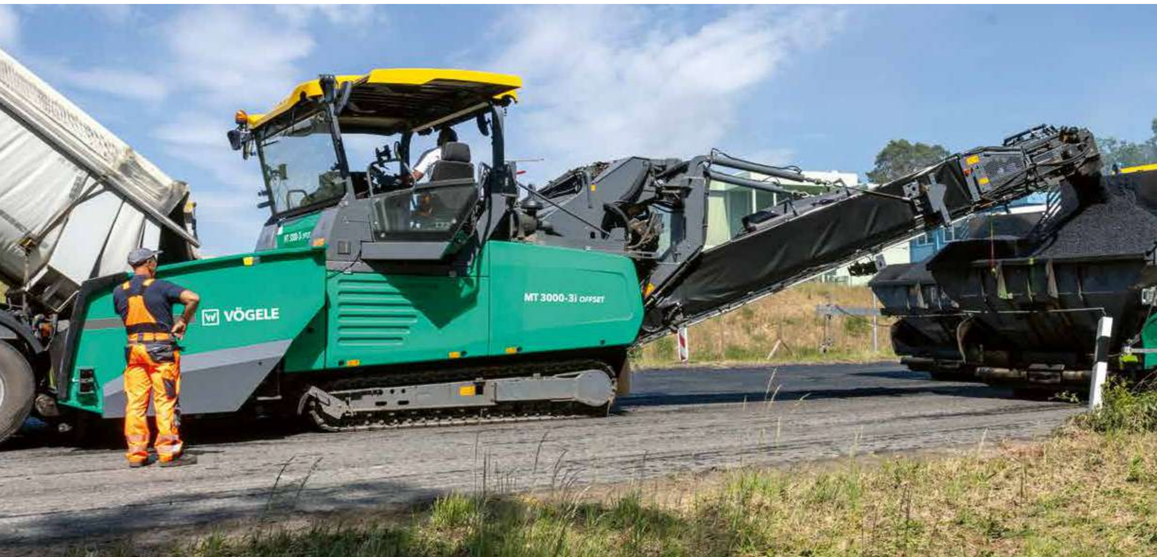
For automatic distance control the operator can select between two different distances.
