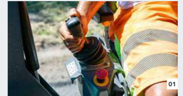
The pivoting conveyor is controlled via a joystick in the armrest of the operator's seat.
