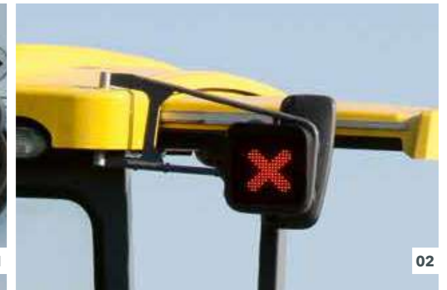
01 Push-button for selecting speed 02 PaveDock Assistant (option)
